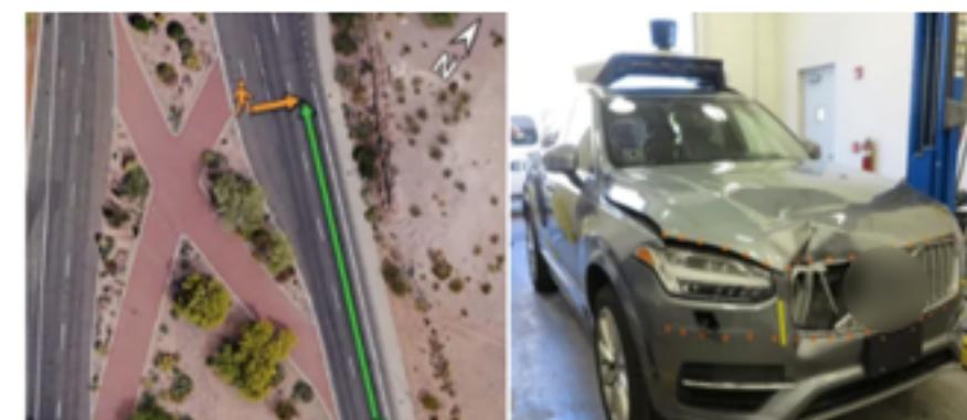
Figure 1. (Left) Location of the crash on northbound Mill Avenue, showing the paths of the pedestrian in orange and of the Uber test vehicle in green. (Right) Postcrash view of the Uber test vehicle, showing damage to the right front side.
